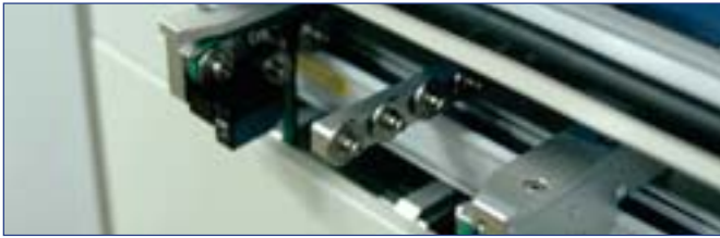
Automatic conveyor width adjustment device and PCB support guide
