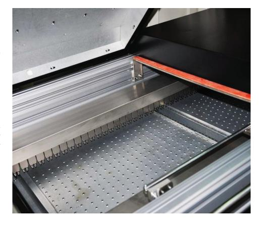
Titanium Finger Conveyor Includes Motorized Width Adjustment and PC Software Control
