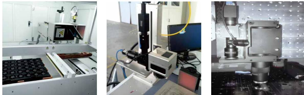
• External coaxial positioning laser marking system • Inner coaxial positioning laser marking system • Paraxial positioning laser marking system
