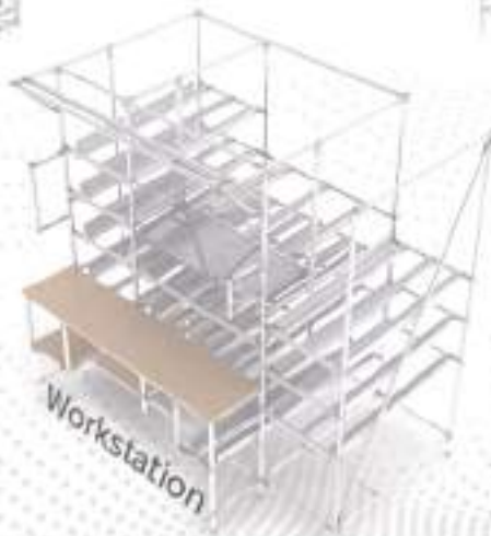
Line Side Rack
